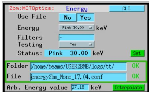
In this example we are setting the DMM to 17.04 keV using the `energy2bm_Mono_17.04.conf` configuration file. Press the “Set” button to move the DMM to this energy.
