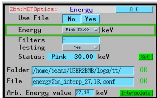
The DMM energy change operates in two modes. The first uses pre-stored energy calibration files. To select this mode set to “No” the “Use File” button:
